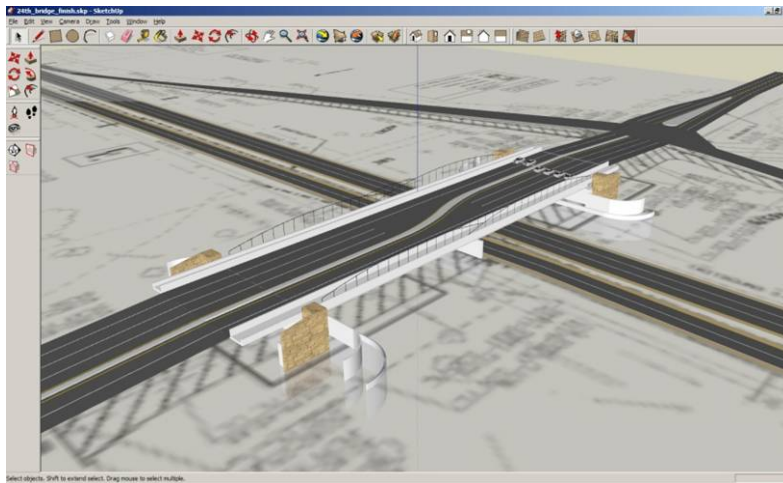
Figure 6. SketchUp purposed bridge model – Created on top of PDF/JPG drawing
