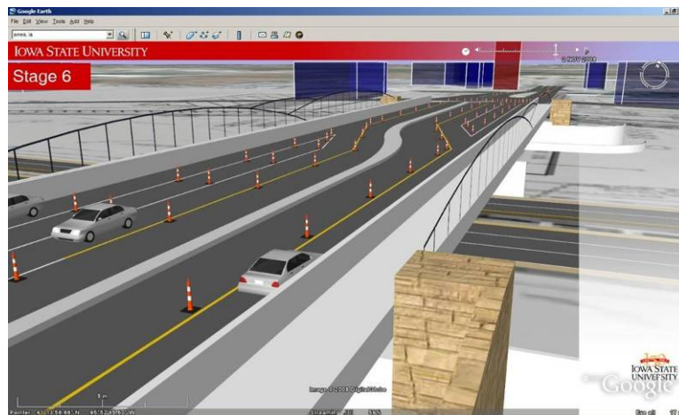
Figure 19. Visualization of 24th Street Bridge northbound during stage 6 displaying in Google Earth
